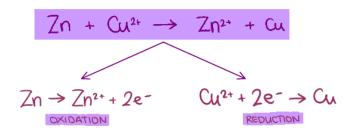
Using these half-equations, it is easy to see where the electron transfer is taking place, and thus determine which species is undergoing reduction or oxidation. The equations must be balanced for the number of electrons being transferred.
