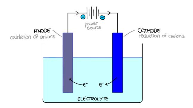
9.5.1 - Describe, using a diagram, the essential components of an electrolytic cell
